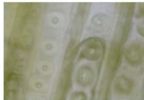
Figure D: Radial View 3 | Additional analyses of the radial face identifies primarily uniseriate bordered pits. The pits are non-aspirated, suggesting the Coastal variety.
